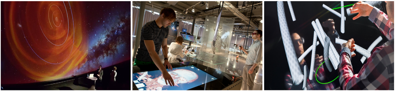
Figure 9: Examples of 3D interaction for knowledge dissemination. From left to right: (a) live presentation in an immersive dome theater using the OpenSpace software [BHY18] for realtime 3D interaction (image © IEEE, used with permission), (b) three scenarios showing volumetric interaction with medical CT data using a touch surface [YRA*16], haptic feedback, and tangible input devices (image © ACM, used with permission), and (c) gesture based 3D interaction with nano tubes [SHLPF14] (reprinted with permission by IGI Global).
