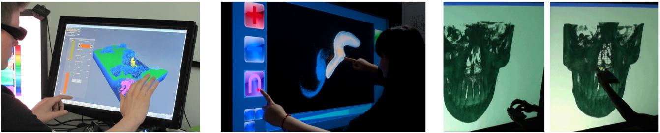
Figure 3: Examples of multi-touch interaction for 3D spatial visualization. From left to right: (a) a seeding point placement technique with a stereoscopic screen [BW11] (image courtesy of and © Thomas Butkiewicz, used with permission), (b) a tactile structure-aware selection technique [YEII12] (image © IEEE, used with permission), and (c) a mobile device's screen used for selection and annotation [SGF*11] (images courtesy of and © Peng Song, Wooi Boon Goh, and Chi-Wing Fu, used with permission).
