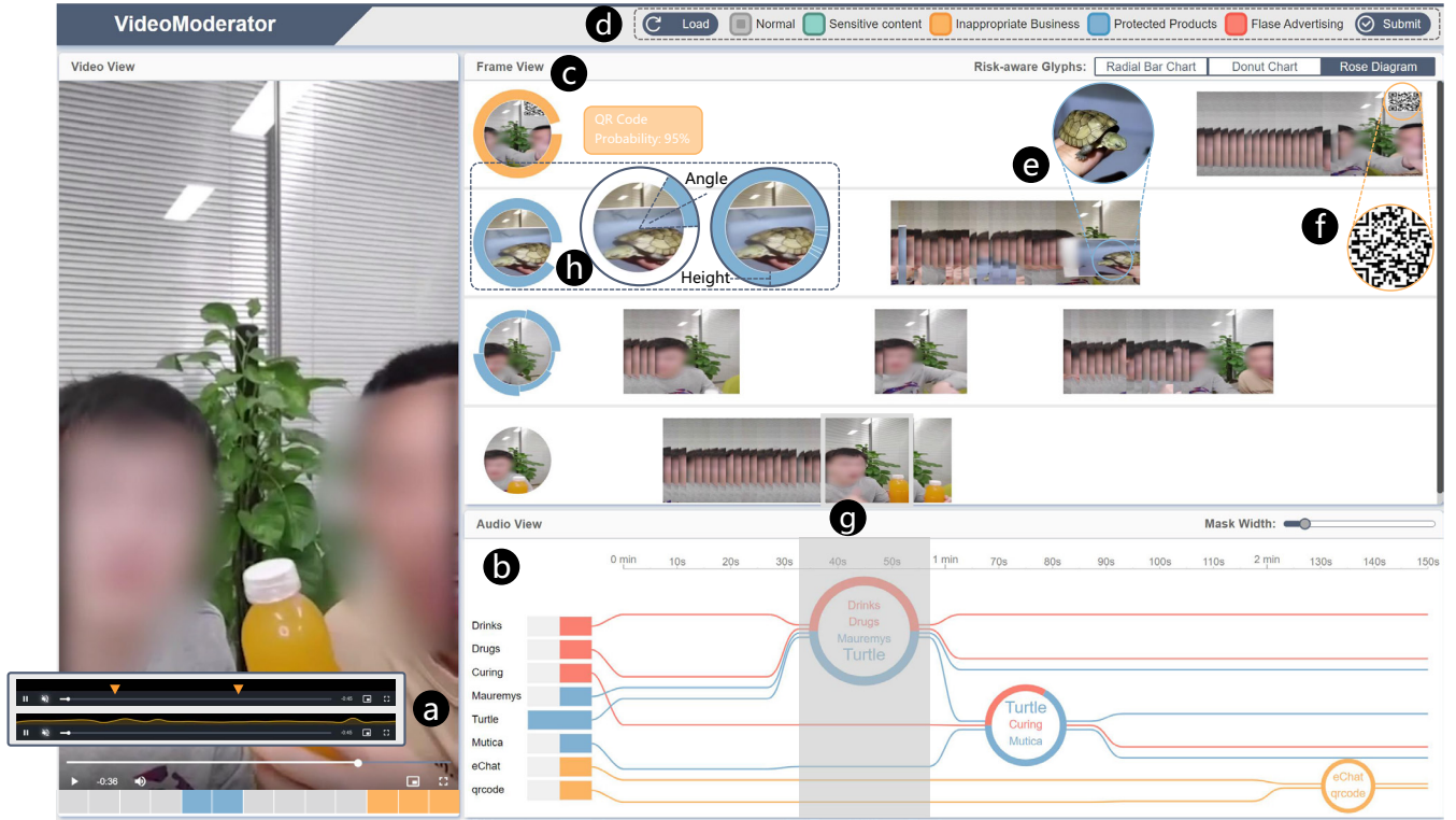
Fig. 4. Multimodal user interface of VideoModerator: (a) a video view with a segmented timeline that demonstrates risk distributions; (b) an audio view with a combination of histograms and a storyline-based words visualization; (c) a frame view that summarizes the video frames; (d) a control panel that integrates a color legend encoding four risk categories; (e) and (f) are discovered insights for video moderation; (g) a moving window that visually associates audio and frame content; (h) circular glyphs that visualize risk-aware information. The dashed lines are manually added.
